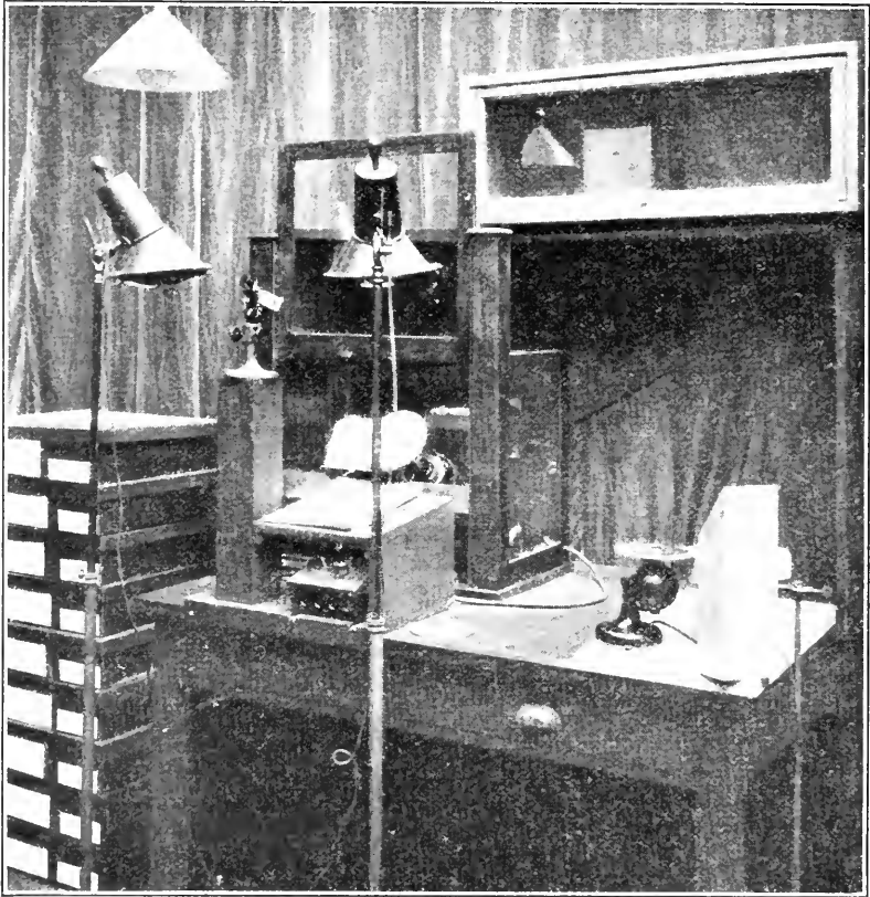
FIGURE 9. First set-up for measuring the color of cotton using a comparator eyepiece. Note that the cotton is in juxtaposition to the color disks and that the lights are so placed as to give a definite angle on the disk surface. This set-up, modified as to the container for the sample, could be used for any other product that presents an even or a nearly even surface for measurement. The equipment has already been used for measuring the color of bread, cheese, condensed milk, and cotton cloth.
